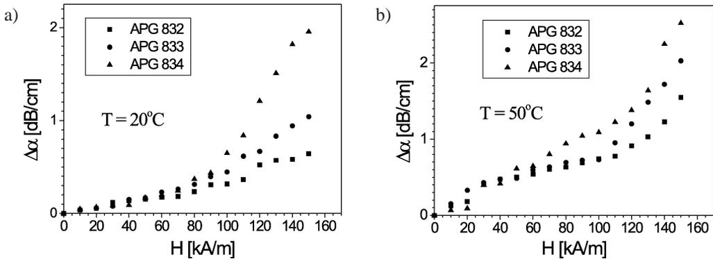
Fig. 2. Changes in the  $\Delta\alpha$  as a function of magnetic field for sweeping time  $t = 10$  min and the temperature: a)  $T = 20^\circ\text{C}$  and b)  $T = 50^\circ\text{C}$ .
