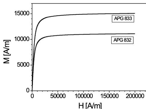
Fig. 4. The magnetization  $M$ , as a function of magnetic field  $H$  for samples APG 832 and APG 833.
