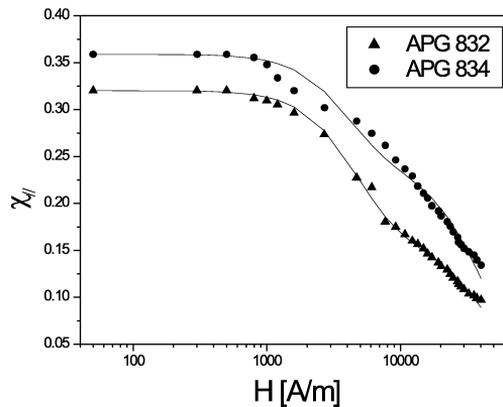
Fig. 5. Experimental values of differential magnetic susceptibility in ferrofluids APG 832 and APG 834 and the theoretical functions best fitting them.
