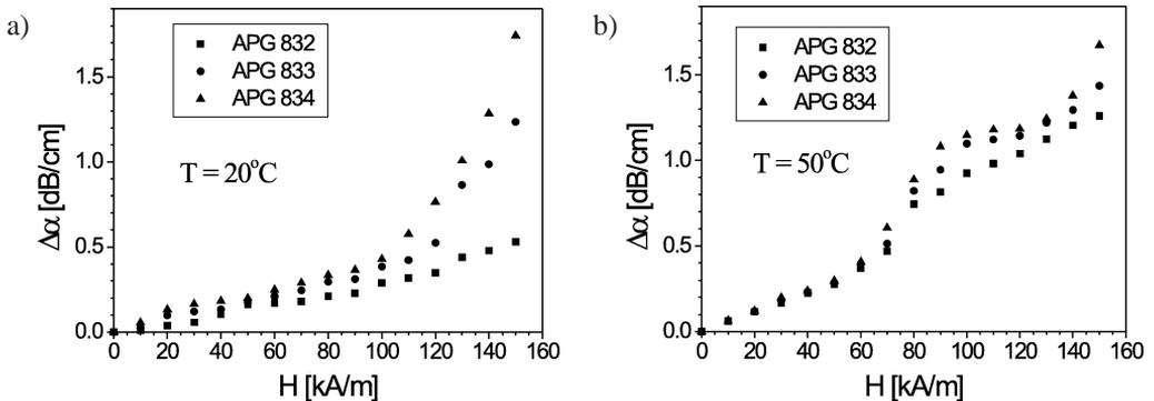
Fig. 3. Changes in the  $\Delta\alpha$  as a function of magnetic field for sweeping time  $t = 5$  min and the temperature: a)  $T = 20^\circ\text{C}$  and b)  $T = 50^\circ\text{C}$ .
