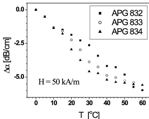
Fig. 1. Ultrasonic wave absorption coefficient changes as a function of temperature subjected to an external magnetic field of 50 kA/m.
