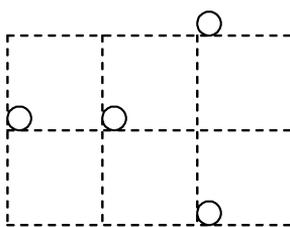
Fig. 3. An antenna array over  $3 \times 3$  grids reconstructed from the array over  $3 \times 4$  grids based on the 2-D GRB  $\{(0, 2), (1, 0), (1, 1), (2, 2)\}$ .
