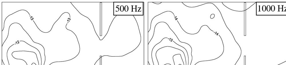
Fig. 4. A distribution map of the influence function for 500 Hz and 1000 Hz for a mechanical workshop.
