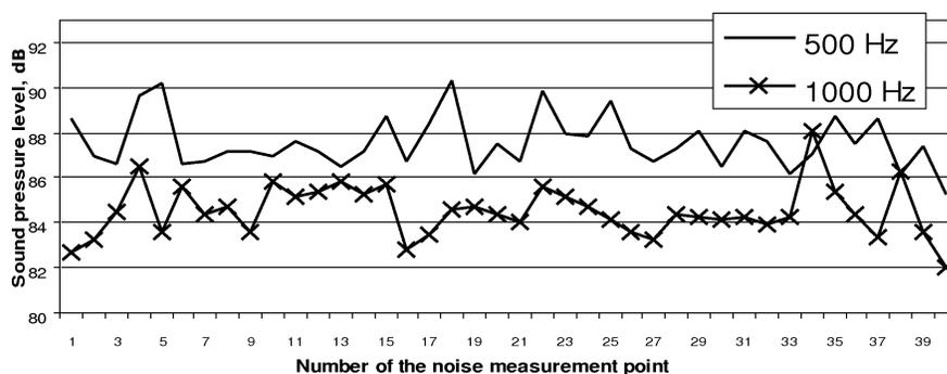
Fig. 5. Fluctuation of the sound pressure level at the source (the grinding machine).
