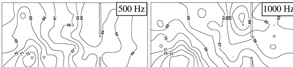
Fig. 2. The distribution of sound pressure levels, determined experimentally, for 500 Hz and 1000 Hz.
