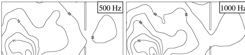
Fig. 3. The distribution of sound pressure levels, estimated in a computer simulation, for 500 Hz and 1000 Hz.
