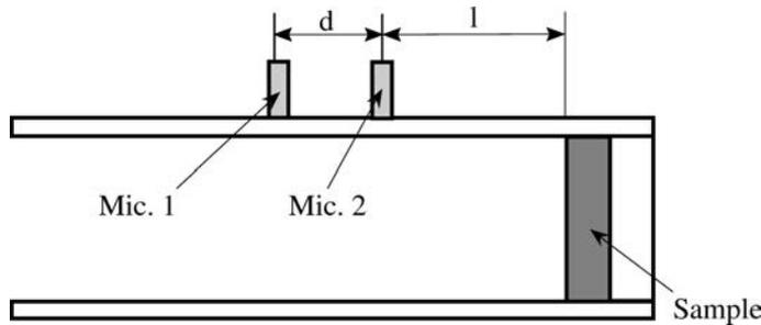
Fig. 1. Experimental setup suggested in the standard ISO 10534-2:1998.
