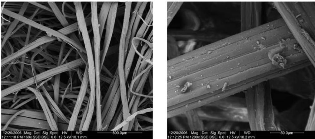
**Fig. 2.** Electron microscopy images of Kenaf wool.
