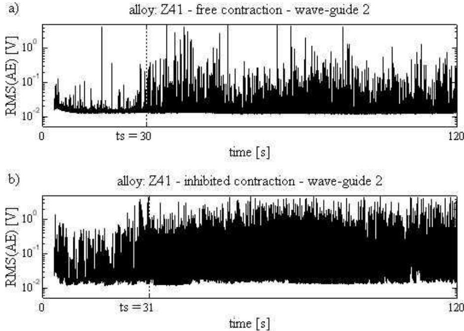
Fig. 2. Envelopes of the AE signal generated during solidification of Z41 alloy castings: a) casting solidifying with a free contraction, b) casting solidifying with an inhibited contraction.  $t_s$  — the end of the solidification.
