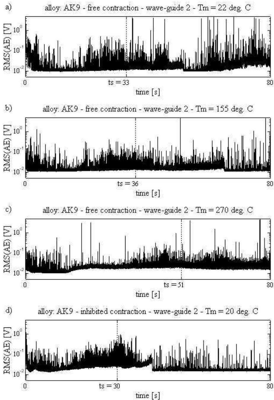
Fig. 1. AE signal envelope generated during solidification of AK9 alloys: a) casting solidifying with a free contraction,  $T_{in.mould} = 22^\circ\text{C}$ , b) casting solidifying with a free contraction,  $T_{in.mould} = 155^\circ\text{C}$ , c) casting solidifying with a free contraction,  $T_{in.mould} = 270^\circ\text{C}$ , d) casting solidifying with an inhibited contraction,  $T_{in.mould} = 20^\circ\text{C}$ .  $t_s$  — the end of the solidification.
