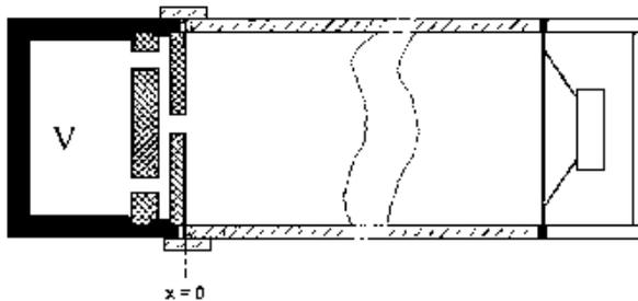
Fig. 1. A resonator of two plates neck mounted in the impedance tube.
