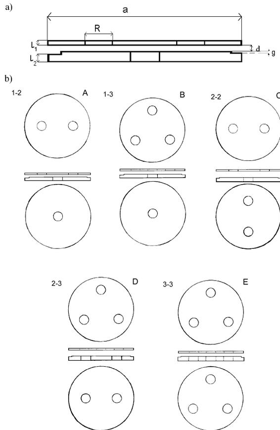
Fig. 2. A configuration of the double cover of the resonator (a) and 5 variants of configurations used in experiments (b).
