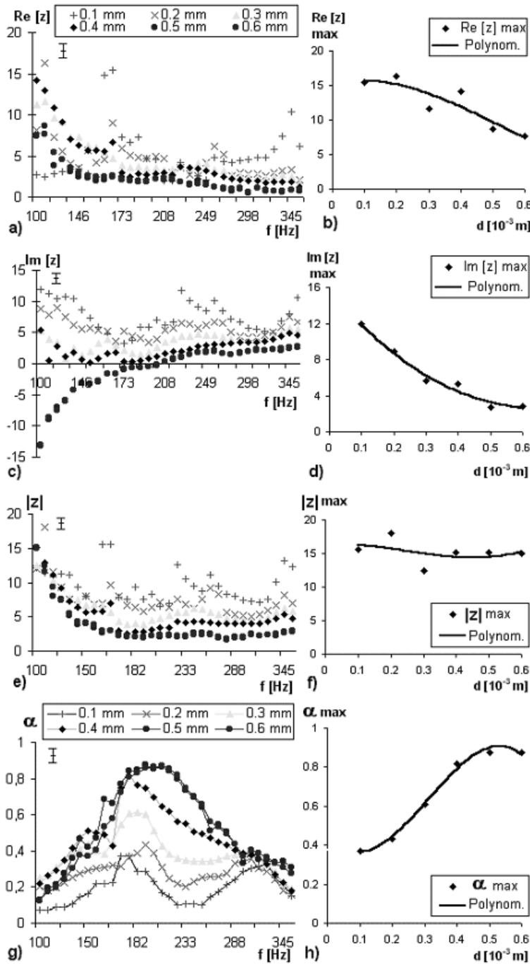
Fig. 4. Dependencies of real  $Re(z)$  (a, b) and imaginary  $Im(z)$  (c, d) parts as well as modulus  $|z|$  (e, f) of acoustic impedance and  $\alpha$  (g, h) against frequency (a, c, e, g) and of their maximum values against distance  $d$  (b, d, f, h) for configuration D 2–3.
