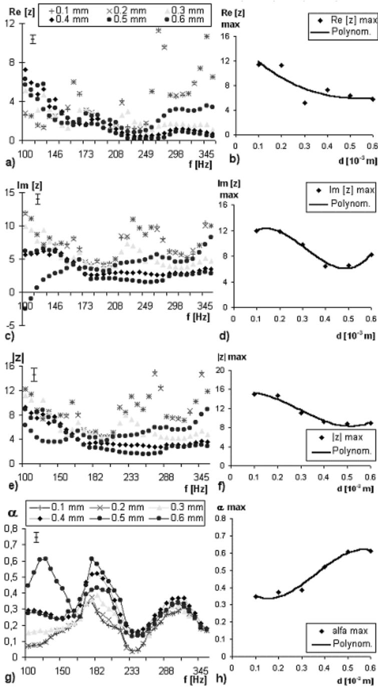
Fig. 3. Dependencies of real  $Re(z)$  (a, b) and imaginary  $Im(z)$  (c, d) parts as well as modulus  $|z|$  (e, f) of acoustic impedance and  $\alpha$  (g, h) against frequency (a, c, e, g) and of their maximum values against distance  $d$  (b, d, f, h) for configuration B 1-3.
