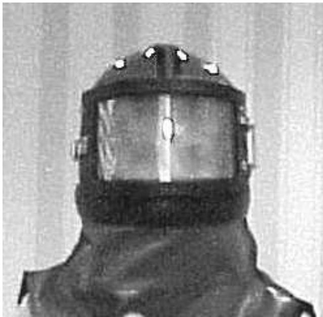
Fig. 1. Shotblasting helmet with panoramic acetate window.
