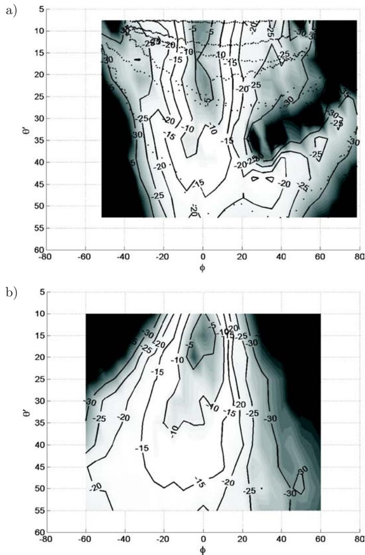
Fig. 6. Comparison between bistatic scattering strengths measured at sea a) and simulated b).
