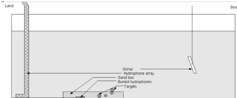
Fig. 4. Full-scale targets are placed in a sand box 10 m (L)  $\times$  5 m (W)  $\times$  0.3 m (D), in the middle of a test basin 80 m (L)  $\times$  10 m (W)  $\times$  8 m (D) later flooded with sea water. The sonar can be tilted to image the targets in the sandbox at different angles of incidence. The hydrophones in the array at the end of the tank allow access to different angles of scattering.
