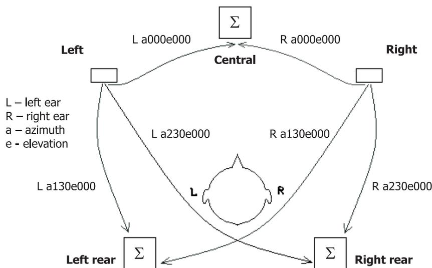
Fig. 2. Signal processing diagram for filtering procedure.
