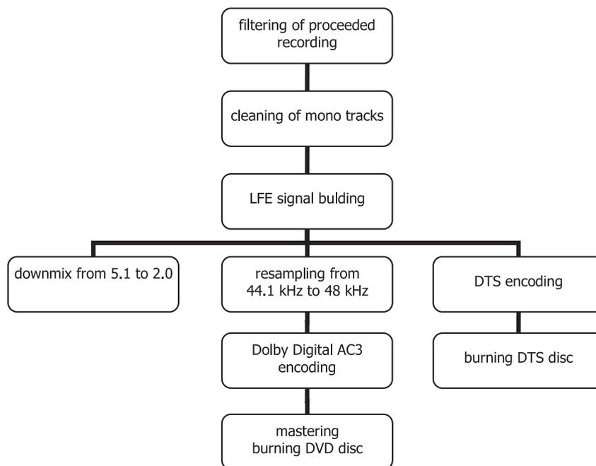
Fig. 1. Block diagram of mix-up process steps.
