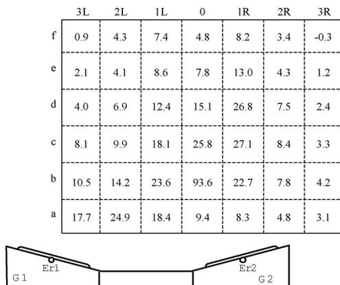
Fig. 3. SPL reduction [dB] of the 250 Hz tone.
