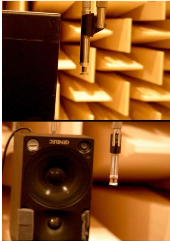
Fig. 1. Genelec 1029A active monitor serving as a broadband monopole source within 50 Hz–2 kHz frequency range next to the Microflown particle velocity sensor.
