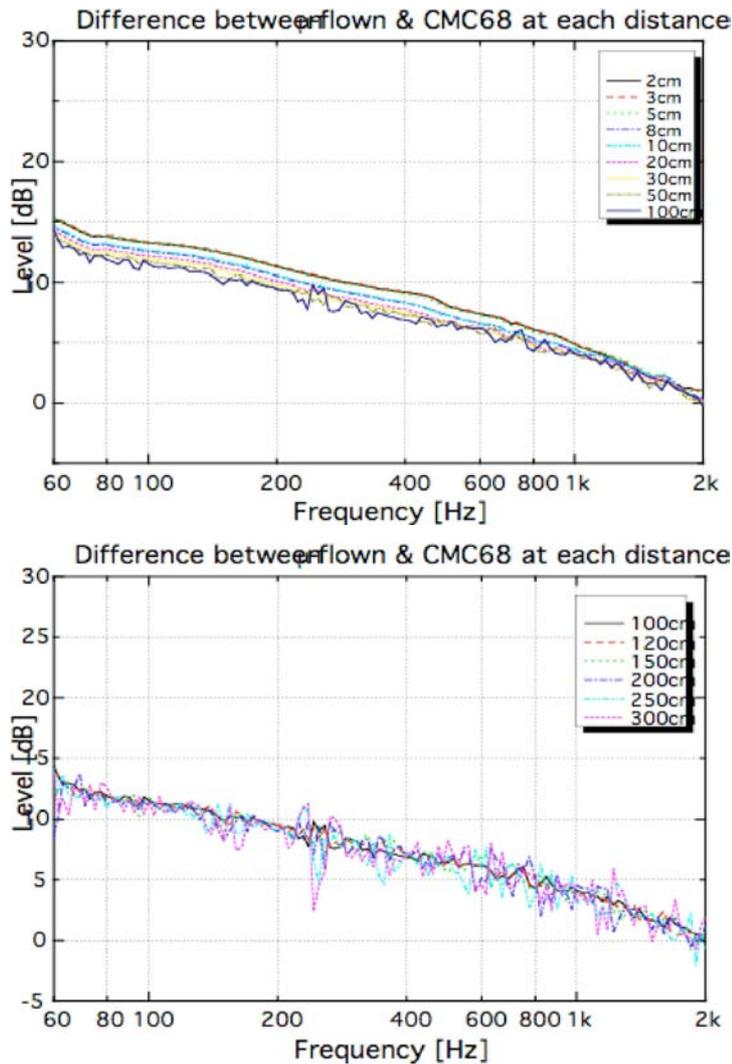
Fig. 8. The difference between the particle velocity and the pressure gradient transducer response at each distance to the source. Distances separated into two graphs: 2 cm – 1 m (top) and 1 m – 3 m (bottom). The average slope is  $-2.6$  dB/oct.
