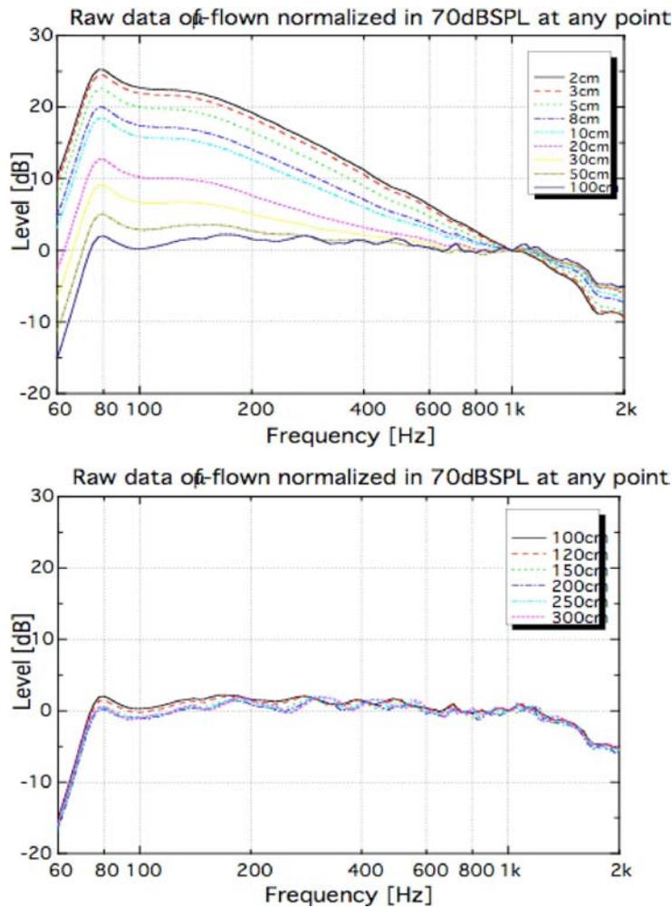
Fig. 4. Frequency response of the Microflow sensor measured using constant 70 dB SPL@1 kHz at each distance, and separated into two graphs according to distance: 2 cm – 1 m (top), and 1 m – 3 m (bottom).
