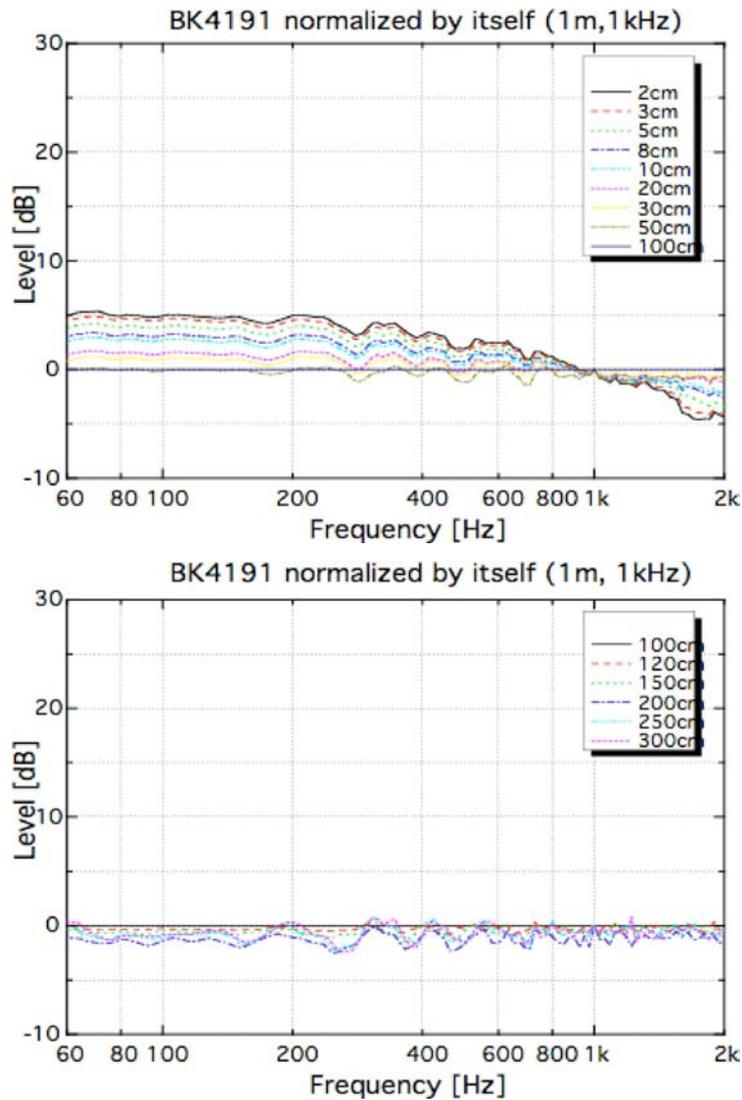
Fig. 9. The frequency response curves of the 1/2'' diameter B&K 4191 microphone measured at various distances to the small sound source and normalized (equalized) with the curve measured at 1 m. Measurements are separated into two graphs: 2 cm – 1 m (top) and 1 m – 3 m (bottom).
