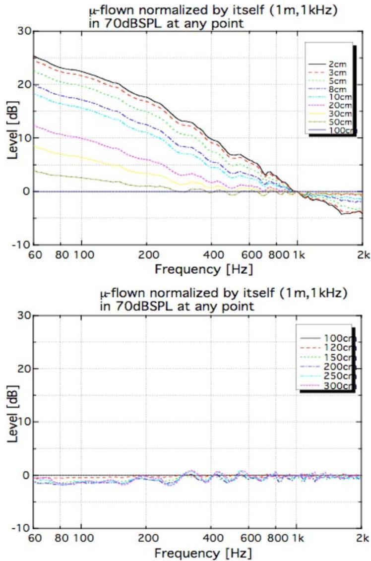
Fig. 5. Frequency response of the Microflown sensor normalized (equalized) with the curve measured at 1 m, and separated into two graphs according to distance: 2 cm – 1 m (top), and 1 m – 3 m (bottom). All curves are calibrated with 70 dB SPL at 1 kHz.
