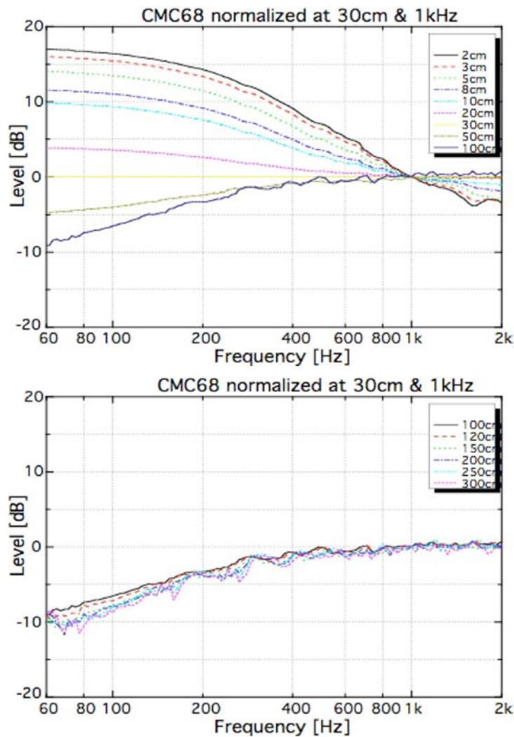
Fig. 7. Frequency response of the Schoeps CMC68 when all response curves are equalized with the flat reference response measured at 30 cm, and matched at 1 kHz. Distances separated into graphs: 2 cm – 1 m (top) and 1 m – 3 m (bottom). Low-frequency roll off affects sources being further away than 30 cm.
