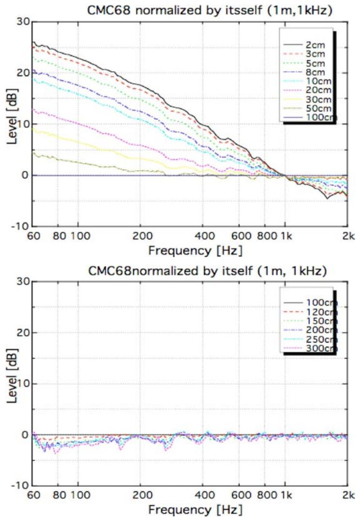
Fig. 6. Frequency response of the Schoeps CMC68 microphone normalized (equalized) with the curve measured at 1 m, and separated into two graphs: 2 cm – 1 m (top) and 1 m – 3 m (bottom). All curves are calibrated with 70 dB SPL at 1 kHz.
