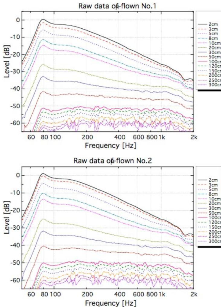
Fig. 3. Frequency response of two Microflown sensors measured at 14 distances to the small broadband source in anechoic chamber.
