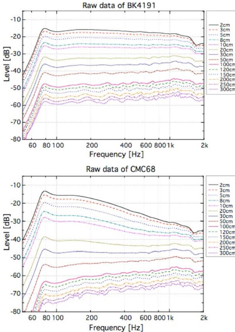
Fig. 2. Frequency response of the pressure (top) and pressure-gradient (bottom) microphones at 14 distances to the small broadband source in anechoic chamber.
