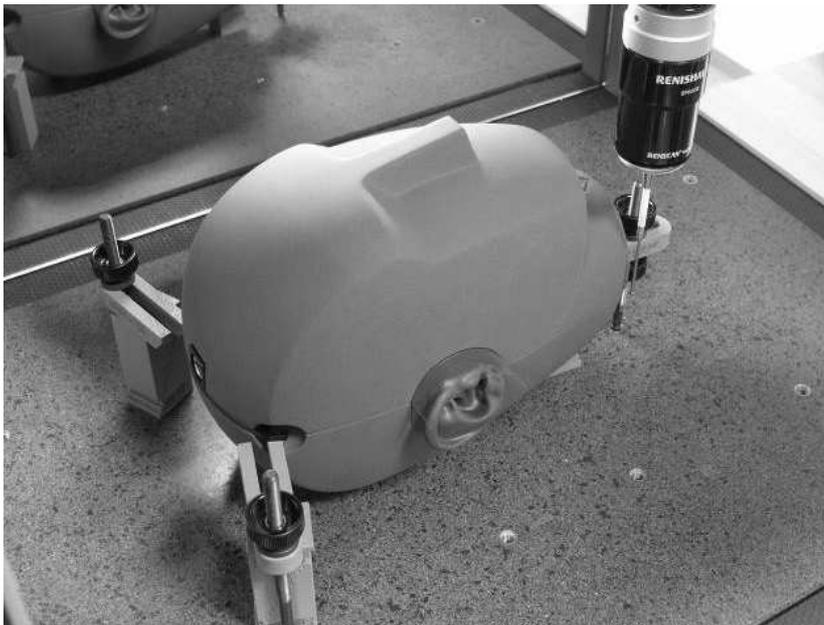
Fig. 3. Dummy head KU 100 in 3-D scanner holder.
