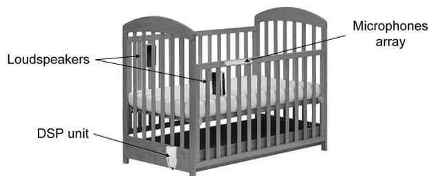
Fig. 1. Contactless hearing aid application.
